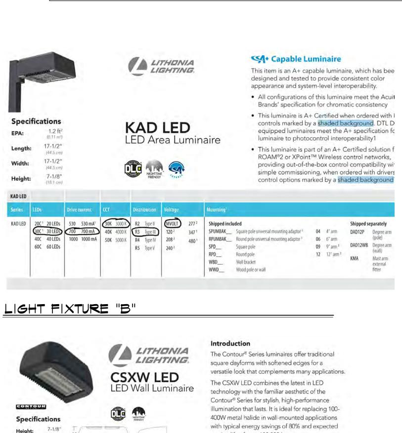
CSXW LED 30C 30 LEDs 700 700 mA 40K 40COK T2M Type II,
