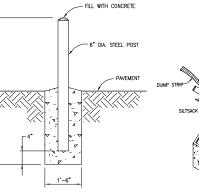
BOLLARD DETAIL (NO SCALE)
