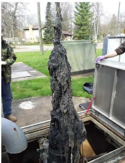
*Pump impacted with flushable wipes.*
