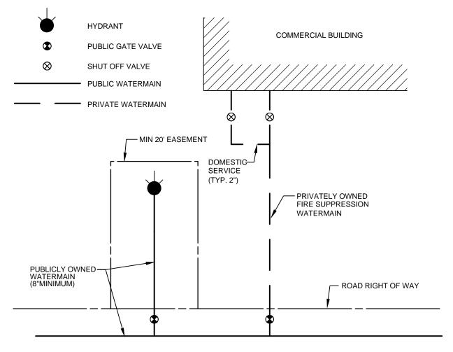
NOTE: FOR FIRE SUPPRESSION LINES, THE MUNICIPALITY WILL ONLY OWN UP TO THE GATE VALVE WHICH MUST BE PLACED WITH IN THE EXISTING ROAD RIGHT OF WAY OR WATER MAIN EASMENT
